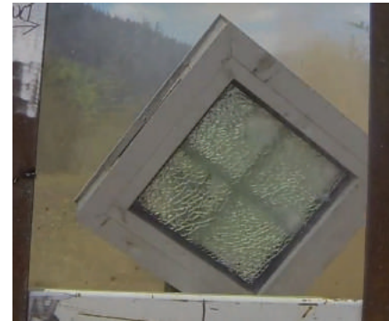
ALUMINUM ALLOY BLAST-RESISTANT WINDOW AFTER EXPLOSION TEST
