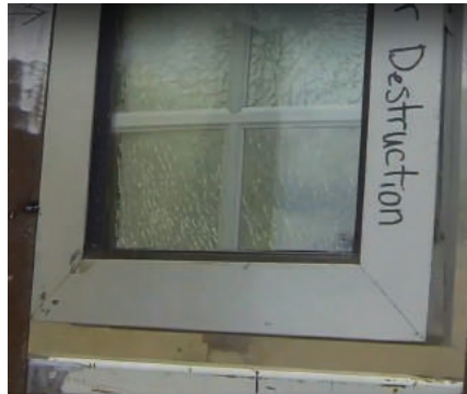
ALUMINUM ALLOY BLAST-RESISTANT WINDOW AFTER EXPLOSION TEST
