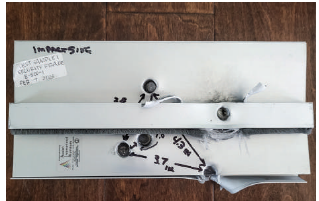
IMPACT SIDE OF SECURITY FRAME SAMPLE AFTER BALLISTIC TEST
